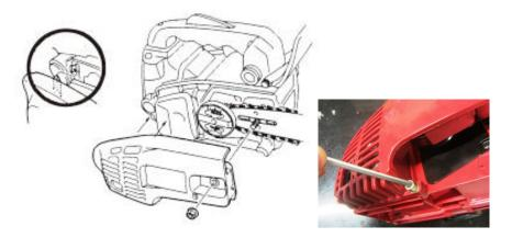
7) Adjust the chain tension by turning the tension screw until the straps touch just the bottom side of the bar.
